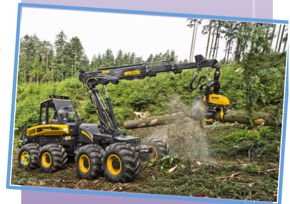
“Harvester” cutting trees to length
