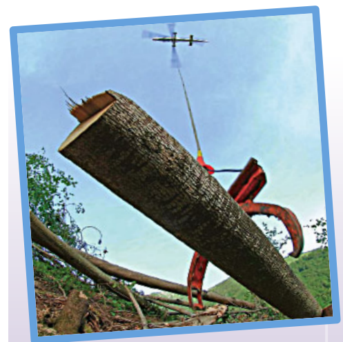
"Grapple Hook" lifting log
