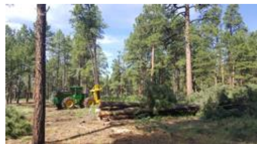
Feller Buncher Cuts and Gathers Small Diameter Trees
